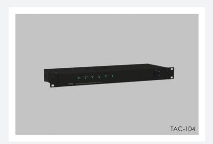
TAC-104 provides supervision of Duty amplifiers and provides automatic changeover of faulty amplifiers to a Standby amplifier. The TAC-104 is capable of monitoring 4 Duty amplifiers with automatic changeover to 1 standby amplifier. The standby amplifier will back-up the duty amplifiers on a first come first serve basis. The unit also provides aural and visual indication to notify users of faulty amplifier.
