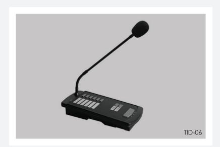
The TID-06 provides 6 loudspeaker zone selection button with ALL CALL, ALL CLEAR and TALK button. LED indicator for chime in progress and ready-to-talk assists the operation of the unit. A BUSY indicator lights when another microphone with higher priority is in use. The remote microphone connects to the Integrated System controller through a single RJ-45 plug and communicates serially up to 1 km. The system is able to handle up to 8 microphones.
